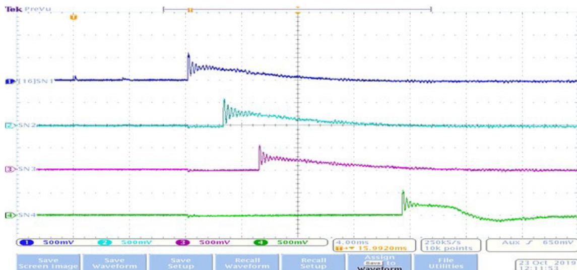
Fig. 4. Shock wave action at 7.5 bar water pressure in three sections
